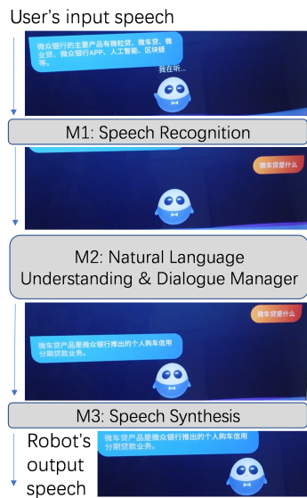
Figure 3: The computational models of robot Xiaowei's dialogue system and corresponding graphic user interface (GUI) design.
